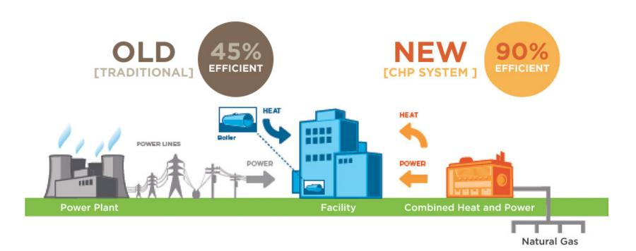
CHP technology takes advantage of the waste heat from electricity production to provide both electricity and useful thermal energy from a single energy source
